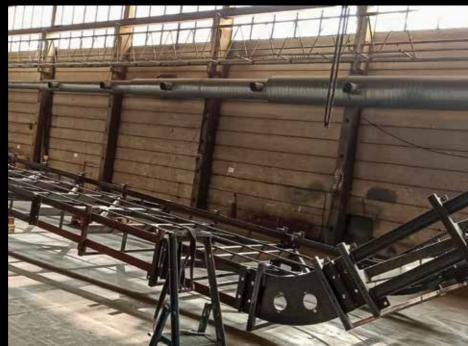
Project: Loaders and unloaders structures City: **Kvänum, Sweden** Year: 2019 – present Type of welding: **135/138** Welding position: PA; PF; PB
